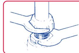
If the premises are occupied or are about to be, pack the dome with Siliphos spheres, replace the filler plug and tighten with the spanner supplied. Turn on the supply and replace the cover, making sure it 'clicks' into position. This opens the valves and allows water to flow. Check for leaks.
