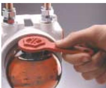
In some cases usage will be such that few spheres are required, even after some time. It is therefore strongly recommended that the entire Siliphos contents are replaced annually irrespective of their apparent condition. Siliphos replacement packs containing sufficient Siliphos to re-fill the unit plus a new 'O' ring seal are available from merchant stockists.
